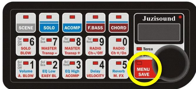
In FAST menu have most common usable parameter, and user need to have fast access to this parameter at any time, by simple pressing one button. Every pressing of button (changing parameter status) will be indicated on display with two consecutive strings. Every strings are show for 1 second. After this, display will be return to string "Fun", to indicate MIDI system current mode.
